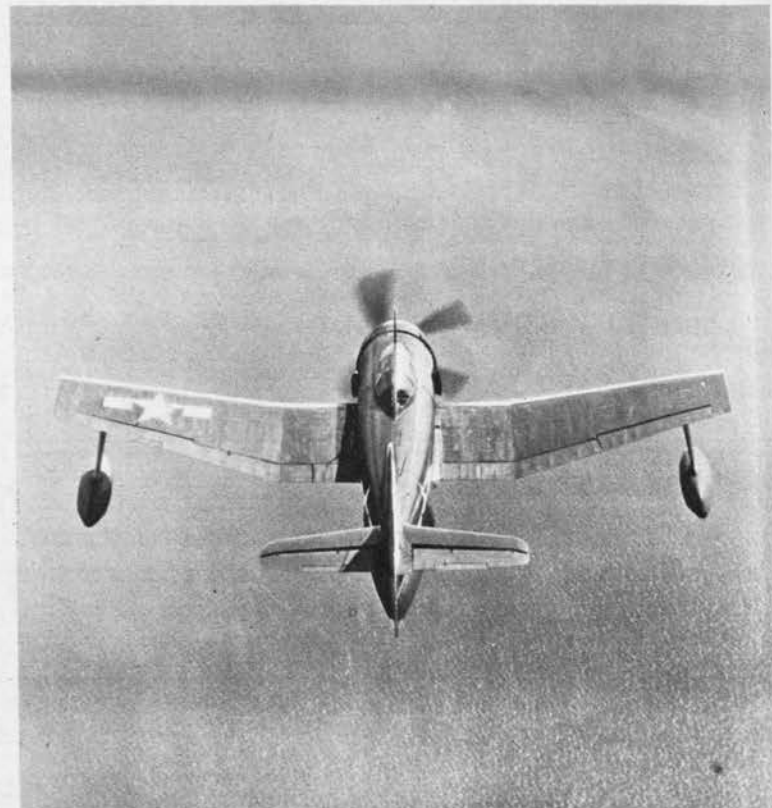
Sharp dihedral of outer wing panels gives SC-1 a distinctive head-on, tail-on appearance. The cockpit canopy forms a conspicuous blister.
